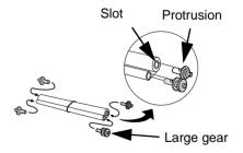
8 Insert the large gear into the large holder on the imaging film cartridge (make sure it clicks into place), and then insert the small gear on the other end of the spool into its holder.
